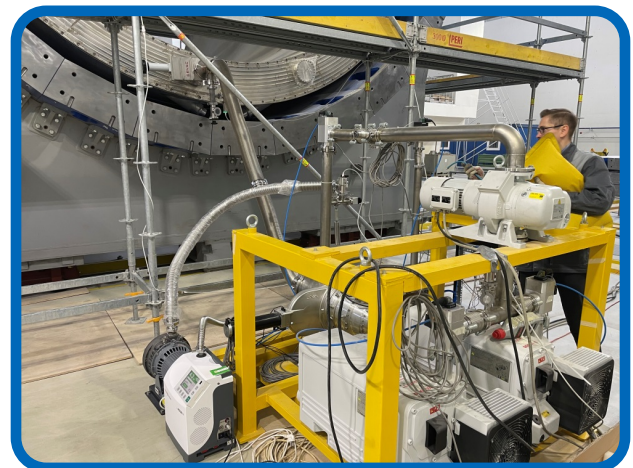
Fig. 6. Testing and tuning of the vacuum solenoid system.
