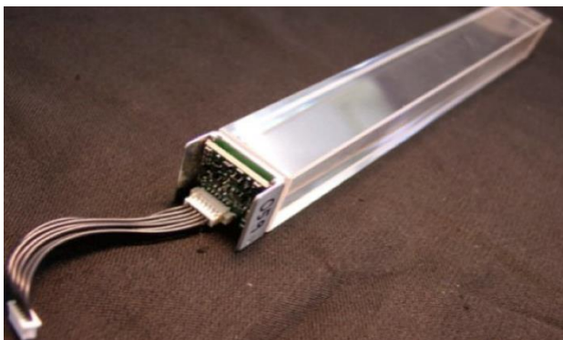
Fig.12. Photodetectors and crystal \text{PWO}_4 with avalanche photodiode.
